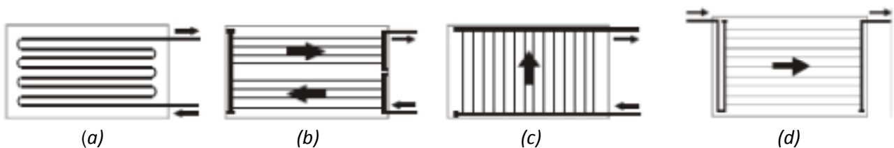
Fig. 8.2.2. Examples of collector design with good emptying behavior. Arrows indicate flow direction at normal operation [3].
