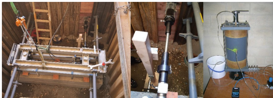
Fig. 4 Press device for in situ push-through tests (left), pull and push coupling of the DH pipes with the press device (middle), Re-SIST shear test device for laboratory investigations (right) ( Source own images )
